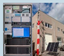
REMOTE - Standalone Solar and Wind powered measuring Unit with Weather station. Where no other electricity supply is available.
