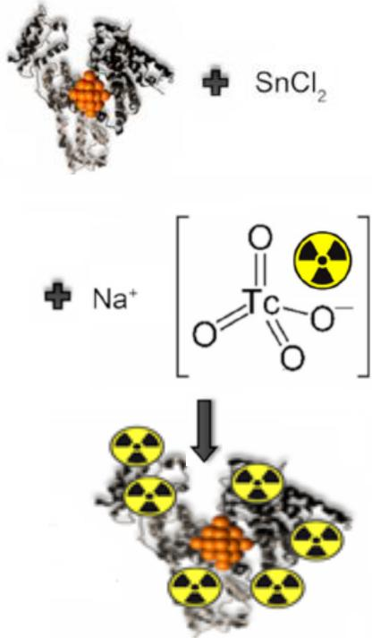
Diagram for the radiolabeling of gold nanoclusters with technetium-99m
