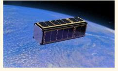
The Trisat-R, the latest Slovenian satellite was successfully launched into space from French Guiana on the VEGA-C rocket on 13<sup>th</sup> of July. Its main purpose are measurements of ionising radiation in the medium Earth orbit to model the magnetospheric environment and better understand space weather.
