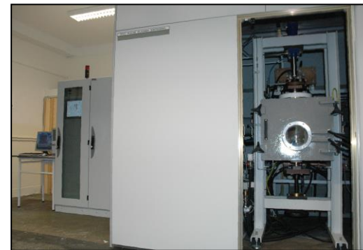
Device for sintering powders using the PPS pulse method (Pulse Plasma Sintering)
