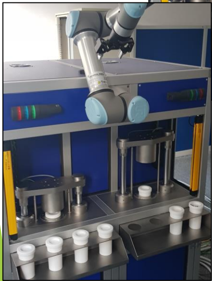
Chemical reactor for microwave hydrothermal synthesis of nanopowders
