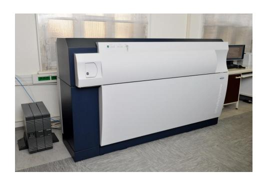
Matrix-assisted laser desorption/ionisation time-of-flight mass spectrometer
