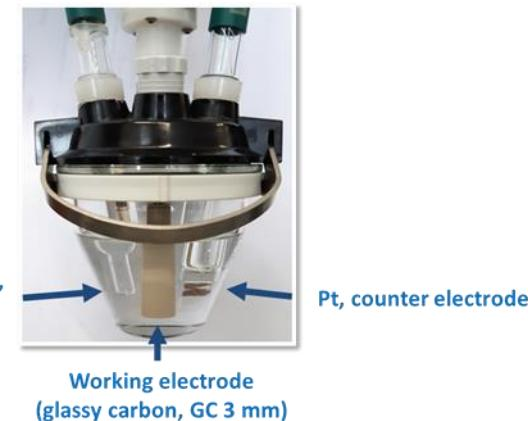
Figure: A three-electrode setup used for electrochemical measurements
