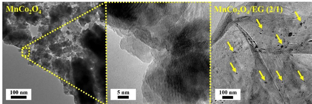
**Figure:** HRTEM images of  $\text{MnCo}_2\text{O}_4$  and  $\text{MnCo}_2\text{O}_4/\text{EG}$  (2/1)
