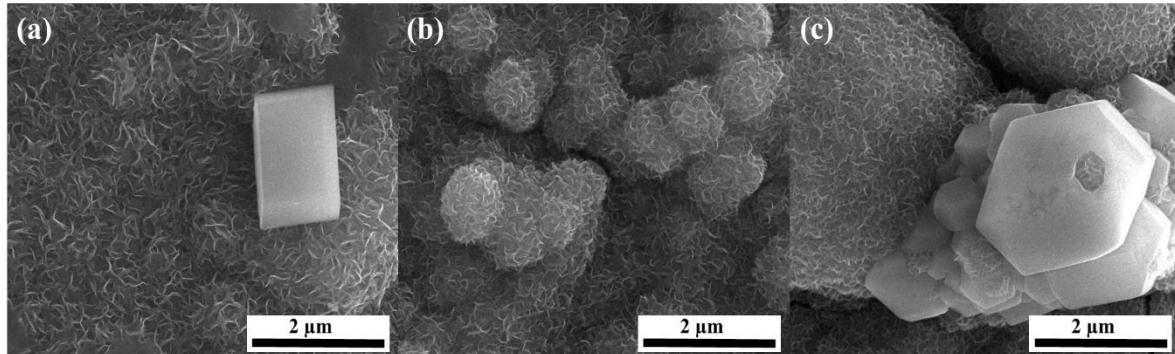
**Figure:** SEM images of samples: (a)  $\text{TiO}_2/\text{SrMoO}_4$ , (b)  $\text{TiO}_2/\text{CoMoO}_4$ , (c)  $\text{TiO}_2/\text{SrMoO}_4/\text{CoMoO}_4$
