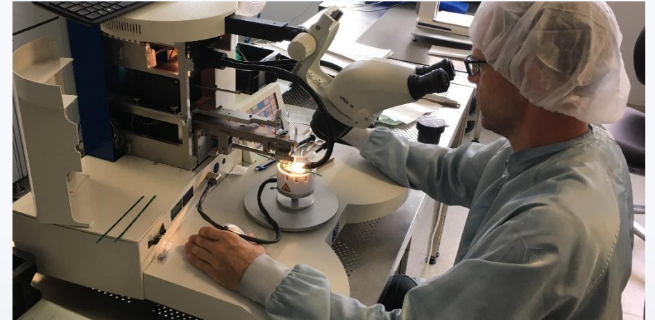
Wire bonding - post processing of samples at RLS d.o.o.
