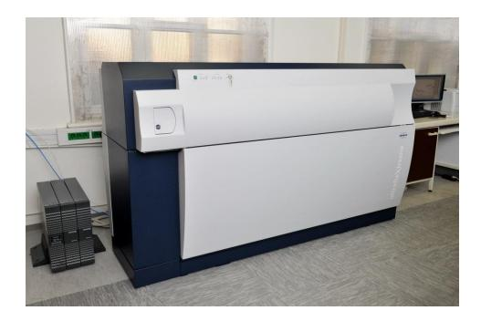
Matrix-assisted laser desorption/ionisation time-of-flight mass spectrometer
